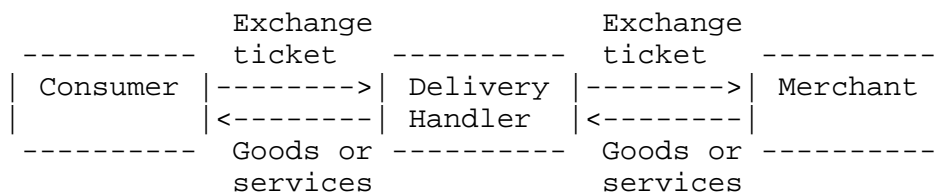
Figure 3. Coordination of untrusted participants using exchange ticket
